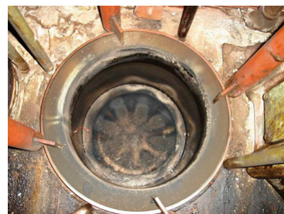
View of damaged cylinder liner with piston fitted.
