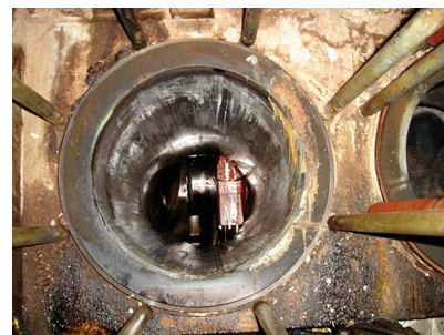
View of damaged cylinder liner.
