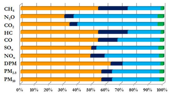
Figure 3.6: 2010 Ocean-Going Vessel Emissions by Mode, %
