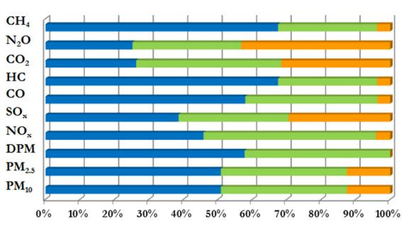
Figure 3.5: 2010 Ocean-Going Vessel Emissions by Engine Type, %
